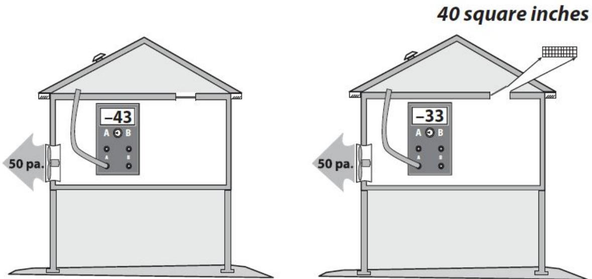
**Formula:** opening area (sq.inch) x factor from table = leakage (CFM50)
